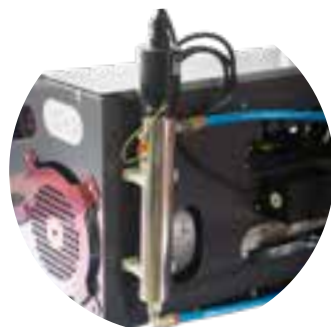
Detail of the sterilising lamp
